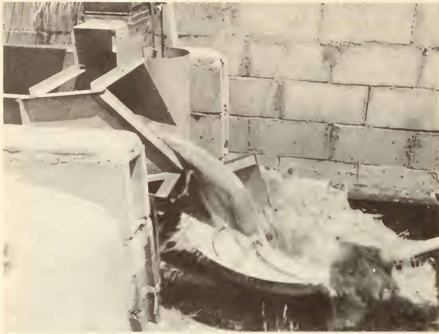
Figure 4.--Soil and water from the runoff plot has passed through the H-flume and is pouring onto the rotary Coshocton wheel, which is taking a sample of 0.5-percent of the runoff with suspended load. This fraction is diverted to the 54-cubic-foot storage tank below the measuring device.
